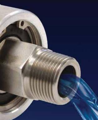
The NEW DWA Series Rotary Union from Duff Norton is designed for use in general purpose, moderate temperature water applications. Other solutions or oils may be used if they are non-corrosive to aluminum and compatible with nitrile rubber. The pipe plug installed in the end of the standard joint may be replaced with special elbows available from Duff-Norton to install either stationary or rotating siphon pipes for dual flow applications.
