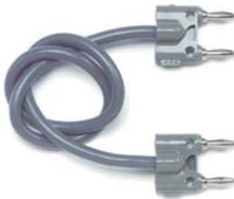
**CAB-023:** Cable Set, Low Thermal EMF Retractable Banana. The CAB023 is a low thermal EMF retractable sheath banana plug patch cord set. These low thermal cables minimize thermal errors so accurate low voltage measurements can be made. Each set includes 2 test leads (one black and one red).
