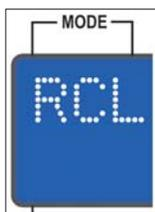
Recall (RCL) - Indicates 526 is in the recall mode. All front panel controls are inactive, except for [LOCAL] key, [UPDATE] key and the SELECTOR knob. Turn the SELECTOR knob will change desired memory location to be recalled.
