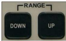
When pressed, the 526 output range will increment or decrement the output to the next range. Selectable ranges are 100mV, 1V, 10V and 100V; 10mA and 100mA.
